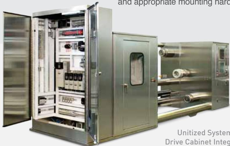
Unitized System with Drive Cabinet Integrated on Machine Frame
