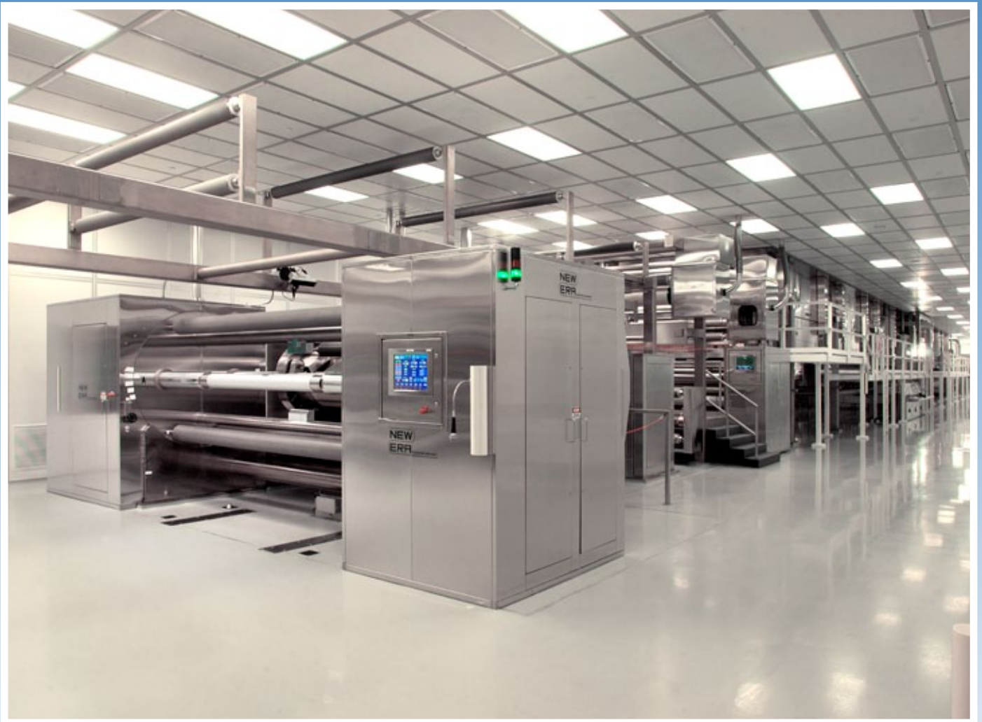
Wide Width, Two Station Cleanroom Coating/Laminating Line
