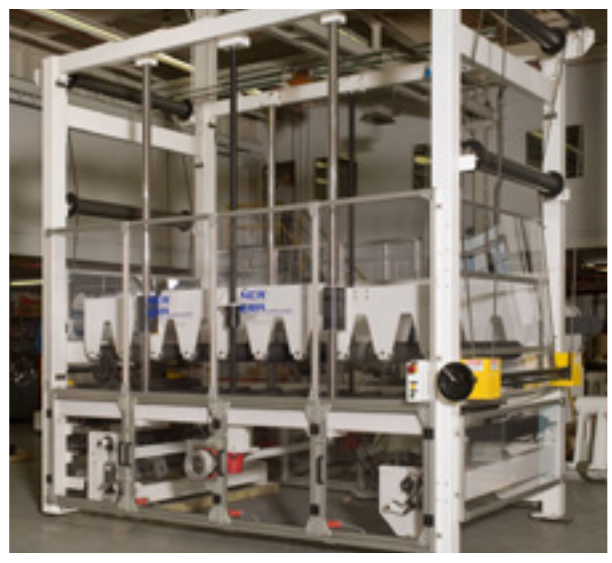
Straight Through Lacing Accumulator
