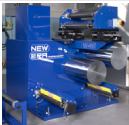
Narrow Width Cooling Station with Oven Exit Guide
