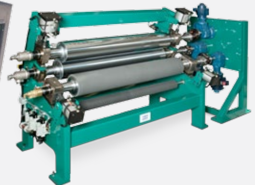
Reverse Roll Coater With 0.000050" TIR Rolls
